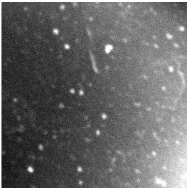
Fig. 1. SEM of Au nanoparticles on graphite (20 keV, 50 kX).
