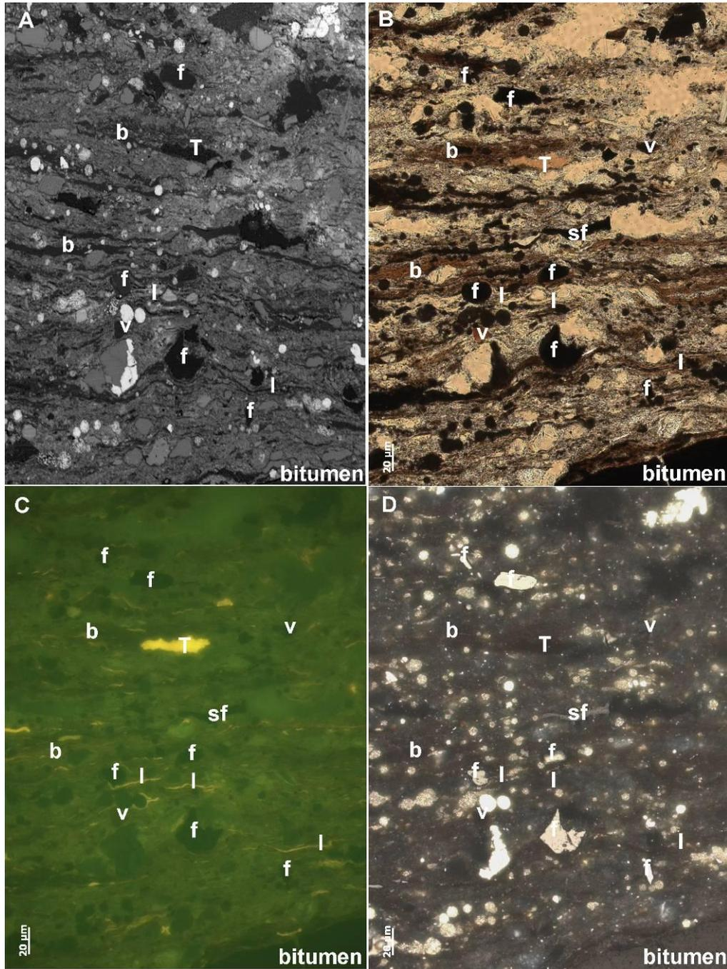
Fig.1. A field of view of a low maturity Kimmeridge Clay Formation sample with a detrital grain of bitumen visible in the bottom of the field. A. backscattered electron image, B. transmitted light image, C. blue incident light under oil immersion, D. white incident light under oil immersion. The letters refer to the identified maceral type: f-fusinite, sf-semifusinite, v-vitrinite, T-*Tasmanities*, b-bituminite, l-lamalginite.
