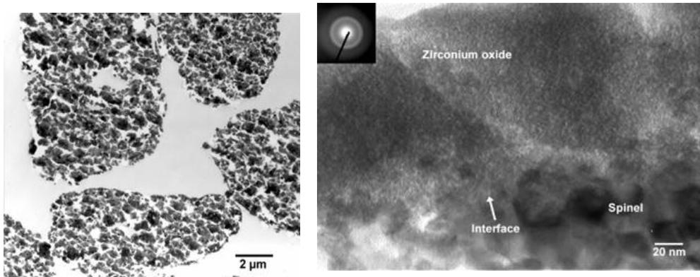
Figure 2. TEM images of ultramicrotomed  $\text{ZrO}_2$ -coated  $\text{LiMn}_2\text{O}_4$  electrode particles, showing amorphous  $\text{ZrO}_2$  layer over  $\text{LiMn}_2\text{O}_4$  particles.
