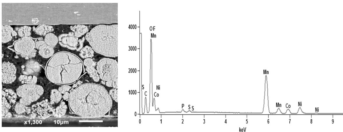
Figure 3. SEM/EDS results from an ion-milled cross-sectioned cathode laminate. The ion-milled surface reveals the internal particle microstructure.
