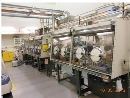
Figure 1. Post-Test Facility argon glove boxes. Cells are dismantled on the right-side glove box, analysis conducted on the left-side glove box.
