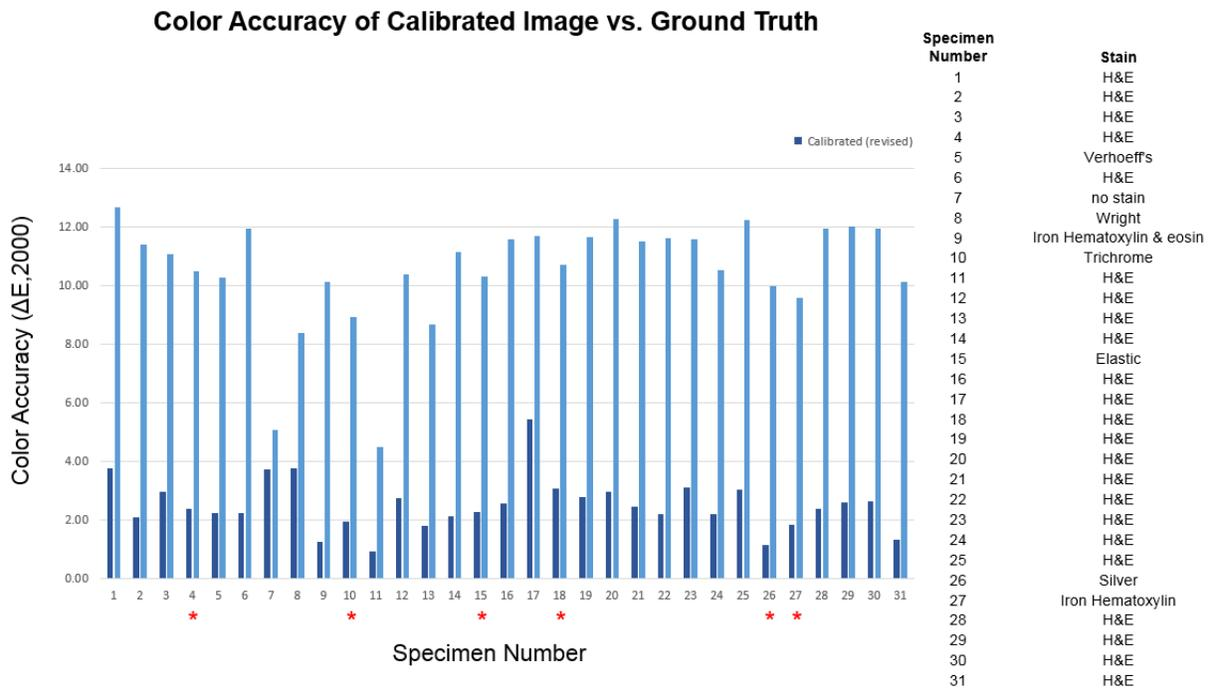
**FIGURE 2:** Color accuracy reported as  $\Delta E$  for 31 specimens representing 9 different histological preparations. Light blue bars indicate the  $\Delta E$  for the RAW images vs. the Ground Truth reference images. Dark blue bars indicate the  $\Delta E$  for the calibrated images vs. the Ground Truth. Specimens denoted with red asterisks (\*) were selected for visual comparison as illustrated in Figure 3.
