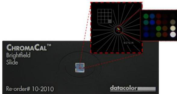
**FIGURE 1:** Depiction of the Datacolor ChromaCal color calibration slide. The central area of the slide houses the calibration chip that consists of two color matrices (one with 30 $\mu$ m circles and one with 9 $\mu$ m circles), and a micrometer grid. The color circles serve as color standards and are described as narrow band, interference-type filters with measured optical characteristics. The neutral-color circles are used to determine the linearity of the image.
