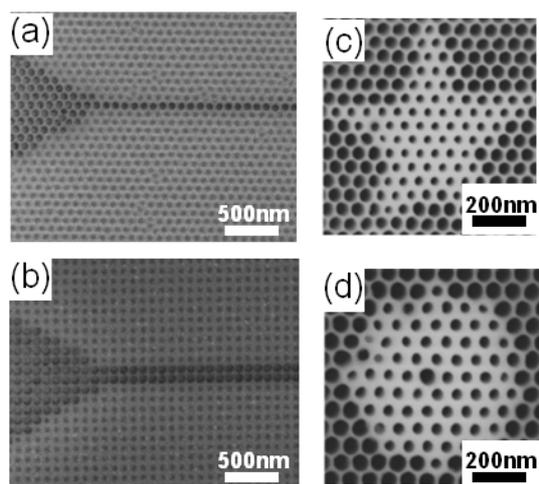
**Figure 2.** (a) Nanostructures with one pore wide, (b) two pore wide, (c) custom-designed star shape, and (d) hexagonal shape.
