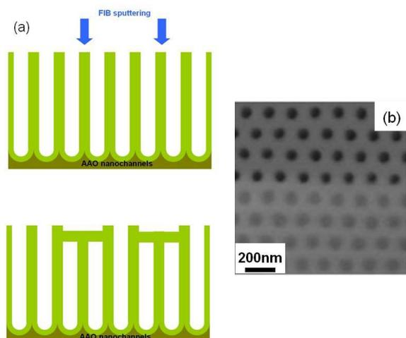
**Figure 1.** (a) Schematic picture showing the process of selective closing AAO nanochannels in an array. (b) Array before (upper) and after (lower) FIB closing.
