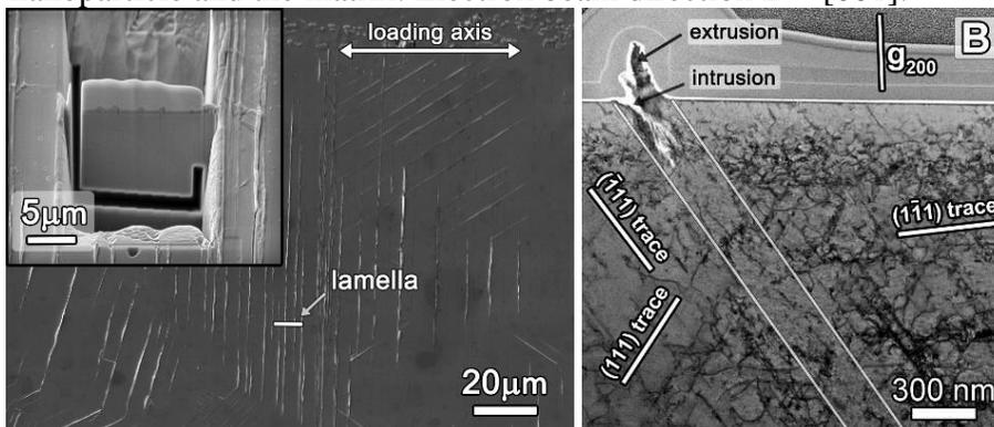
**Figure 3.** PSBs and the position of the lamella within the grain. On the right is an image of the PSM B consisting of extrusion and intrusion and a crack starting from the intrusion. Dislocation arrangement in the PSB is ladder-like.
