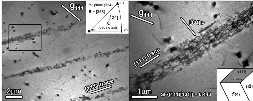
**Figure 1.** Planar dislocation structure consisting of dislocation rich bands where dislocation rich walls and dislocation poor channels alternate. Mostly edge segments of primary dislocations with Burgers vector  $1/2[1\bar{0}1]$  are visible.
