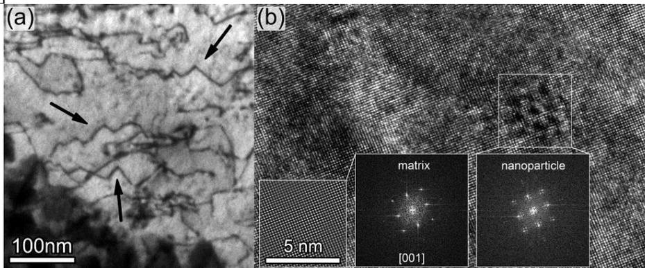
**Figure 2.** (a) Dislocations pinned by small hardly visible microstructural units. (b) HR-TEM image of nanoparticle in FCC matrix. Comparison of FFT made from the matrix and particle area indicates coherency of the nanoparticle and the matrix. Electron beam direction  $B = [001]$ .
