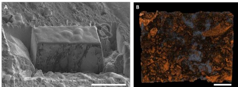
**Figure 2.** FIB-SEM of Bakken shale (A) Backscatter electron image. Scale bar is 20  $\mu\text{m}$ . (B) Segmented porosity image. Scale bar is 10  $\mu\text{m}$ .
