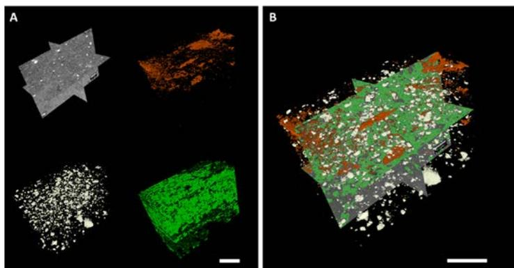
**Figure 1.** CT image of the Marcellus. (A) Orthographic slices through the greyscale CT volume, fractures (orange), heavy minerals (white), and organic matter (green). Scale bar ~0.25 mm. (B) Combined isolated features.
