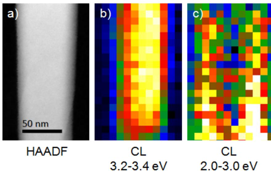
**Figure 2.** (a) HAADF image of a ZnO nanowire. (b) CL map of the 3.3 eV bandgap emission. (c) CL map of the 2.0-3.0 eV defect emission. Each pixel in a CL map contains a CL spectrum; (b) and (c) are generated by integrating the spectra over the indicated energies, and are normalized to each map's maximum intensity.
