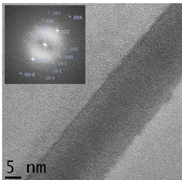
**Figure 1.** HRTEM image of a ZnO nanowire. The inset is the Fourier transform, where Bragg reflections are labeled with the  $hkl$  indices of wurtzite ZnO.
