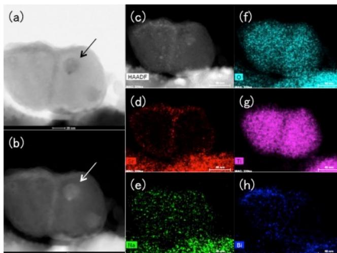
**Figure 1.** Formation of core-shell structure upon calcination at 700 °C. (a) and (b) represent the BF- and DF-STEM images, respectively, of the calcined core-shell structure, indicated with arrows. (c-h) represent the HAADF image and elemental mapping of the particles.
