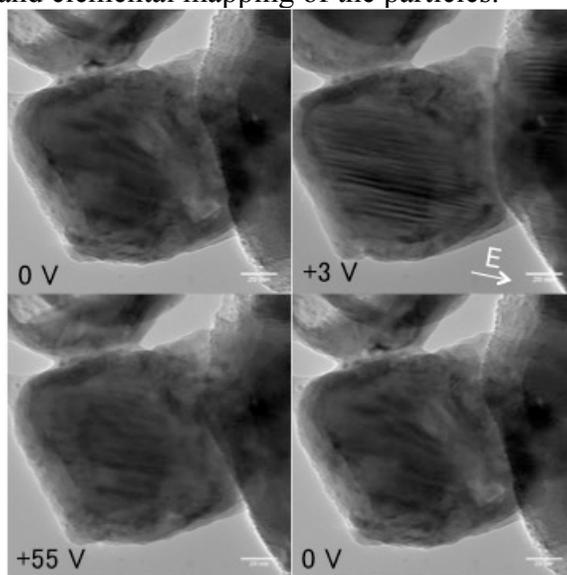
**Figure 2.** Evolution of domains at 700 °C upon application of e-field.
