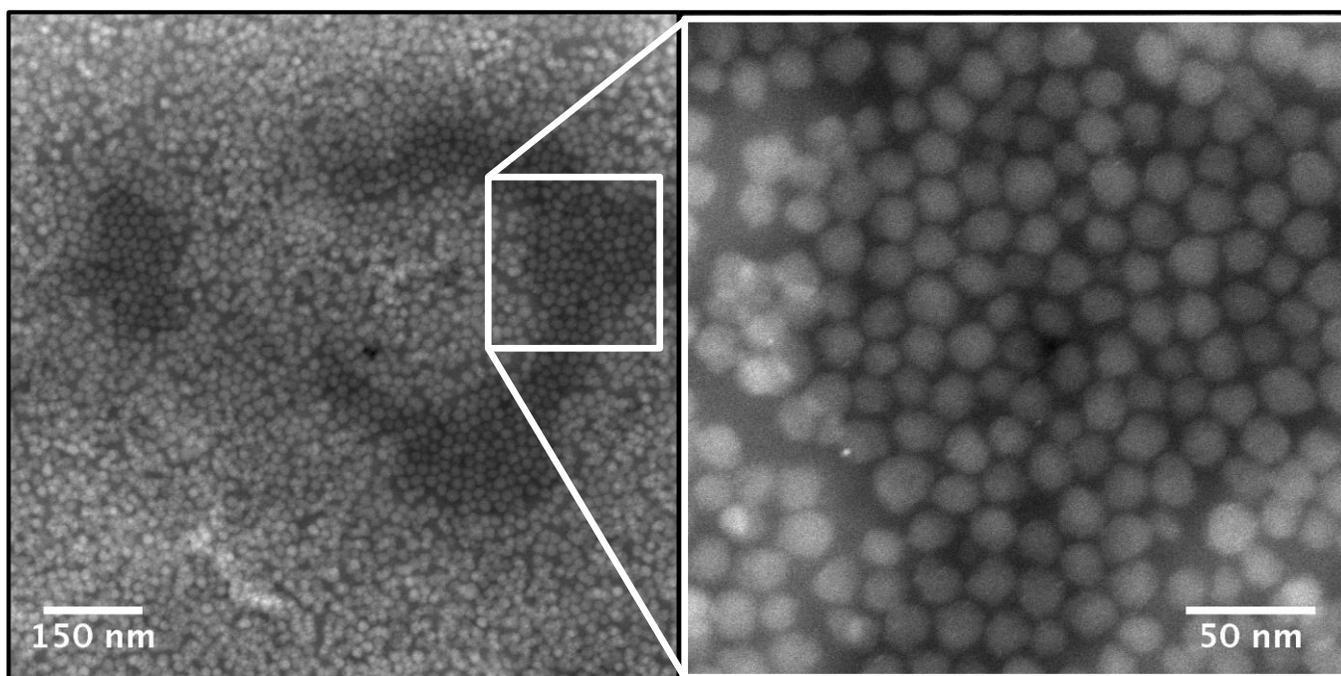
**Figure 1.** Cryo-immobilization of solid/liquid nanostructures by plunge freezing enables high-resolution characterization by cryo-STEM. Cryo-STEM imaging of silica nanoparticles from lithium metal battery hybrid electrolyte, embedded in vitreous ice.
