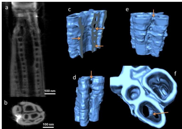
Figure 2. A tomographic reconstruction of TiO<sub>2</sub> nanotubes (a) Longitudinal slice view through the reconstruction (b) Cross-section of the reconstructed volume (c-e) The surface of reconstructed volume after segmentation of selected nanotubes with depicted bridges between nanotubes (f) The surface of reconstructed volume after segmentation of selected nanotubes with depicted place where nanotube split into two nanotubes.
