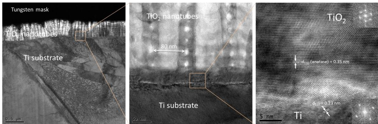
Figure 1. Cross-section STEM images of TiO<sub>2</sub> nanotubes on Ti substrate (a) Overview BF-STEM image of the prepared sample (b) BF-STEM image of TiO<sub>2</sub>/Ti interface region with visible nanotubes walls (c) HR-STEM image of TiO<sub>2</sub>/Ti interface
