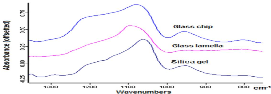
Figure 2. FTIR spectra of glass chip, glass lamella and silica gel.
