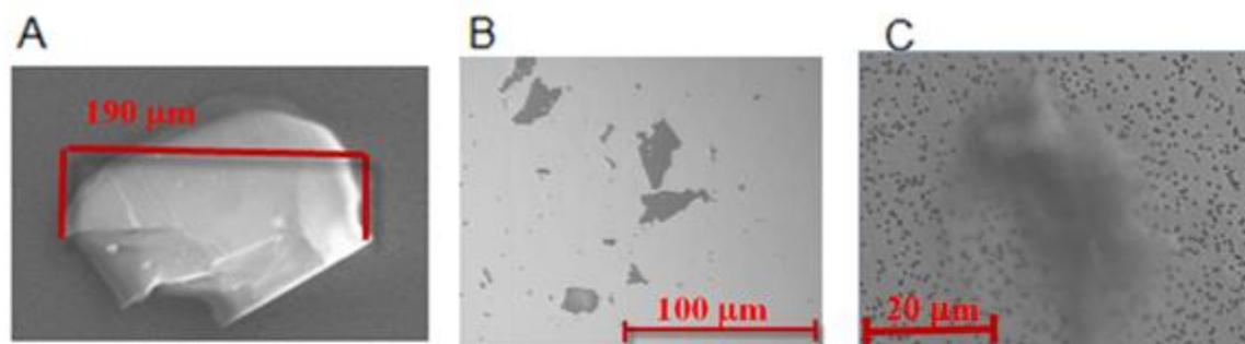
Figure 1. SEM images of a glass chip (A), glass lamellae (B) and silica gel (C).
