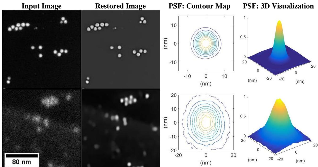
**Figure 1.** Comparison of Aura Processing at Different Beam Energies. The top row of images corresponds to a 20kV beam, while the bottom row corresponds to a 3kV beam. The input image and restored image columns use the same scale bar as shown in the bottom leftmost image. The PSFs show lowest to highest elevations as dark blue to light yellow, respectively.
