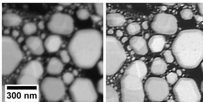
**Figure 3.** 617 Gold Standard. The image on the left was taken with the same operating conditions as the 3kV nanoparticles shown in Figure 1, bottom leftmost image. The image on the right is the restored image, which used the PSF determined for 3kV in Figure 1, bottom rightmost image. Both images shown here have the same scale.
