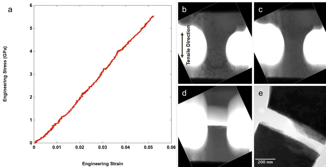
**Figure 1.** Quantitative in-situ TEM tensile test of biotite mica. Loading direction parallel to  $[010](001)$ . (a) Engineering stress-strain curve showing nominally elastic behavior and brittle fracture. (b-d) Still frame images from in-situ video acquired during straining. (b) Sample before loading. (c) Frame before failure,  $\sigma = 5.5$  GPa. (d) Frame after failure. (e) Bright-field TEM micrograph of fracture surface.
