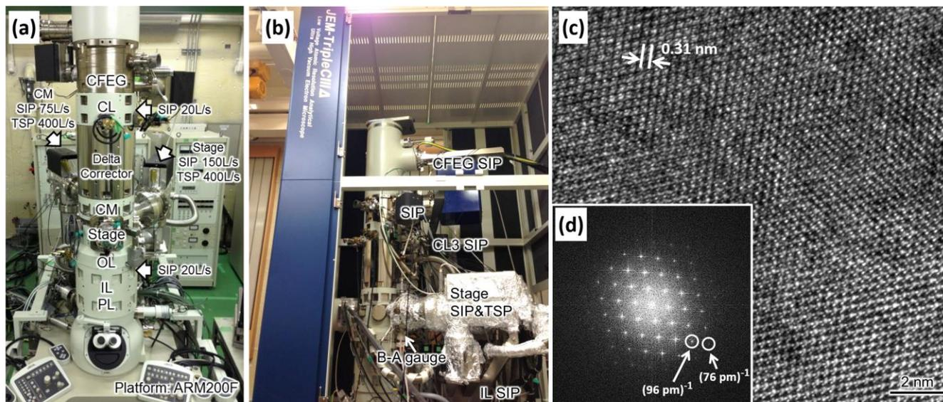
**Figure 1.** (a) and (b) Photos of low-kV UHV STEM instrument (TripleC#3). (c) shows TEM image (without Cs corrector) of Si[110] crystal taken at 60 kV. (d) shows Fourier transform (FT) of the TEM image.
