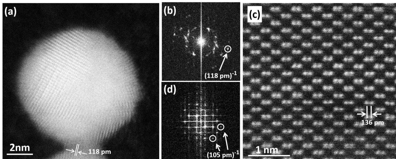
**Figure 2.** (a) ADF-STEM image of gold particle and (b) its FT. (c) ADF-STEM image of Si[110] crystal and (d) its FT. These images were taken at 60 kV with convergence semi-angle of 35 mrad, pixel time of 32 $\mu$ s/pix, and the pressure of stage chamber of  $4 \times 10^{-7}$  Pa.
