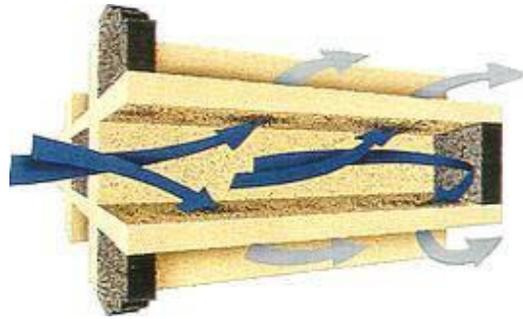
**Figure 1.** A cell of the wall-flow filter (source: Corning)
