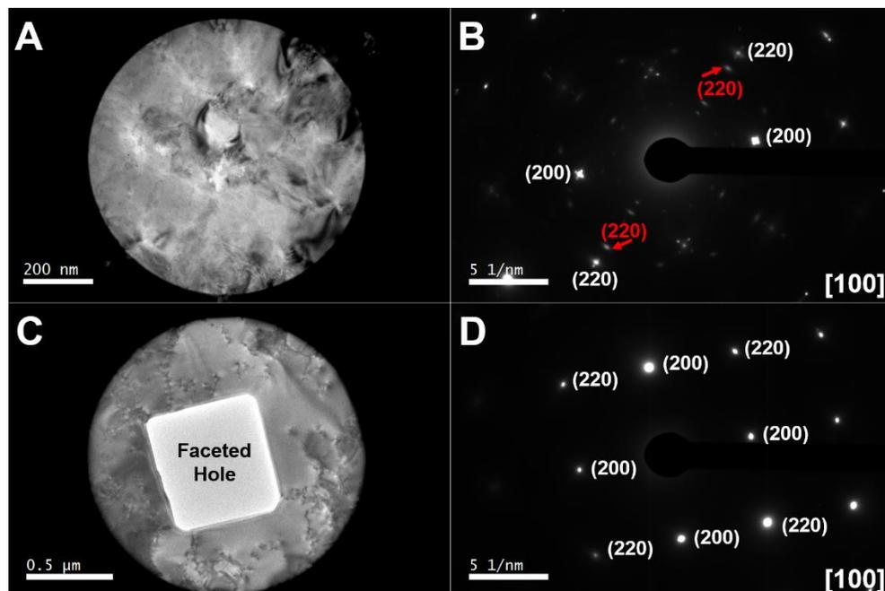
**Figure 1.** Representative bright-field TEM micrographs (A,C) and corresponding selected area electron diffraction patterns (B,D) of a copper film. The *in situ* faceted hole formation and removal of the native copper oxide at 550° C and  $7.6 \times 10^{-4}$  Torr  $H_2$  is highlighted in panels C and D.
