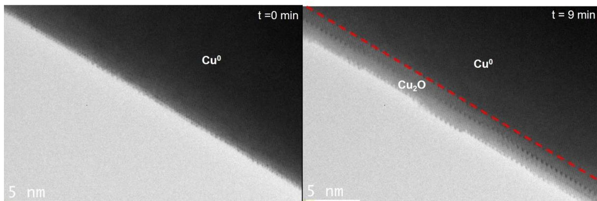
**Figure 2.** *In situ* oxidation of a copper film at a faceted hole. The initial Cu (110) surface prior to oxidation (left) and after 35 mins of oxidation at 250°C and  $1 \times 10^{-5}$  Torr  $O_2$  (right). The red dashed line indicates approximate initial site of the metallic copper facet (right).
