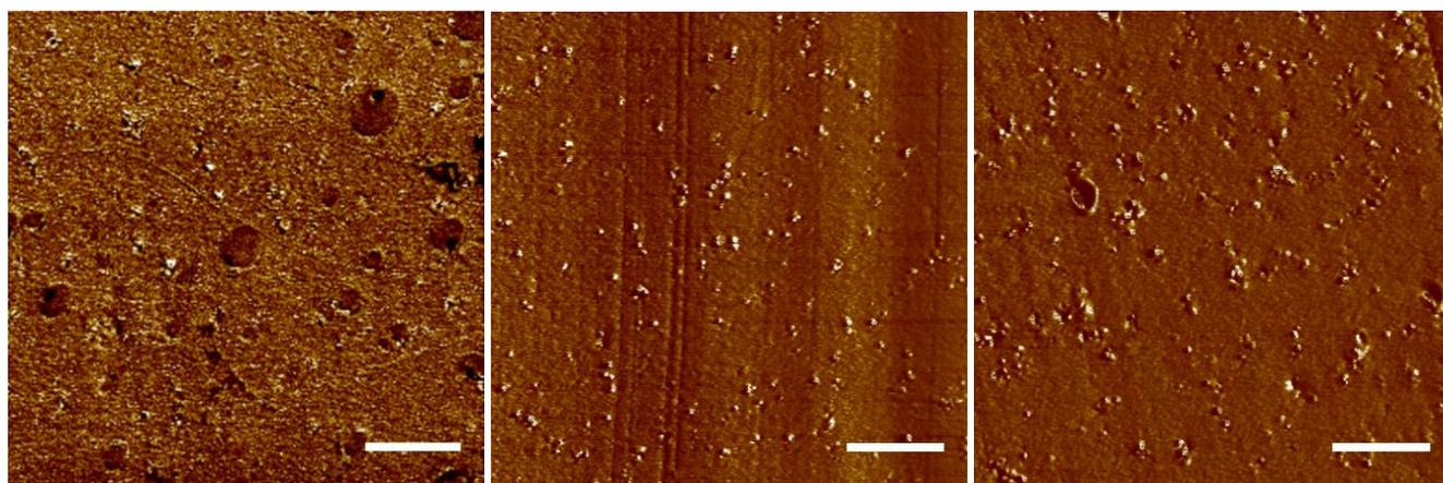
**Figure 1.** AFM modulus map images of ultramicrotome prepared powder coating samples. All additives (right) and individual additives: air-release additive (center) and flow additive (right). Scale bar is 1 micron.
