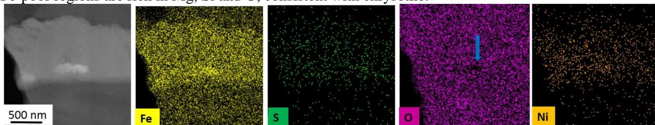
**Figure 2.** HAADF and EDS images of a FeNi oxide grain with an O-poor relict core (blue arrow).
