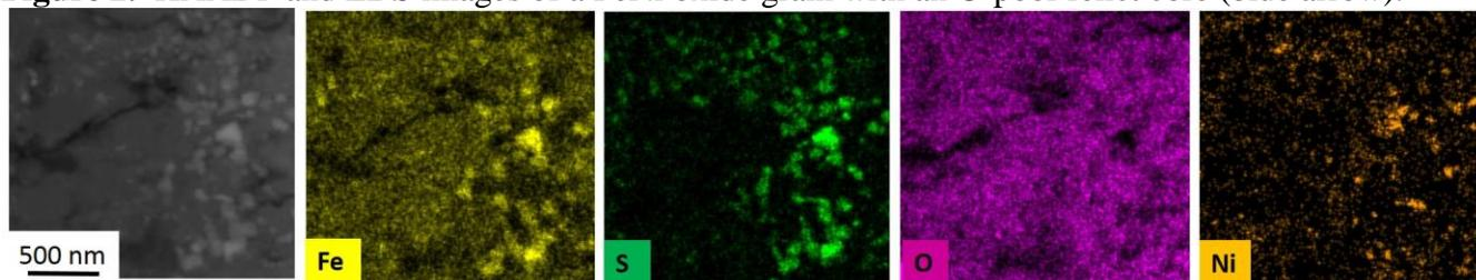
**Figure 3.** HAADF and EDS images of a S-poor conduit present within the matrix (lower right of images). The O-map (pink) shows that the Fe-sulphides are O-poor and Ni-rich.
