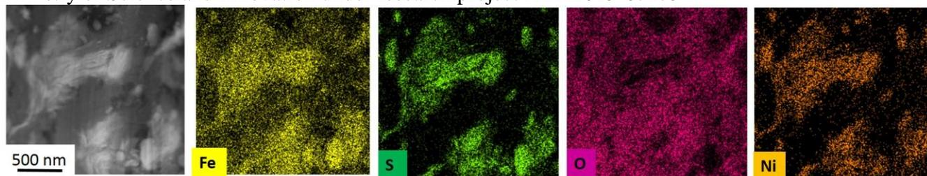
**Figure 1.** HAADF and EDS images of regions rich in Fe, Ni, S and O, consistent with tochilinite. The Fe-poor regions are rich in Mg, Si and O, consistent with chrysotile.
