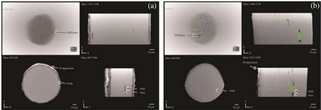
**Figure 1.** PFIB 3D reconstruction of (a) HP Nitinol wire showing the segmentation process. The colored features represent NMIs (pink) and pores (blue) and (b) SP Nitinol wire showing the same segmentation process and colored features representing NMIs (green) and pores (blue).
