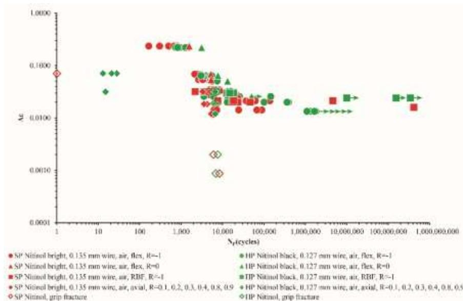
**Figure 2.** Comparison of all HP Nitinol and SP Nitinol fatigue data representing axial fatigue for R = 0.1, 0.2, 0.3, 0.4, 0.8, and 0.9, flex bending fatigue R = 0 and R = -1, and rotating bending fatigue with data points defined as run-out denoted with right-facing arrows and specimens that broke at/near the grip indicated with open diamonds
