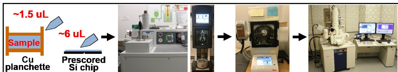
Figure 1. Illustration of cryogenic scanning electron microscopy specimen preparation method: Sample application, freezing, etching, and observation.
