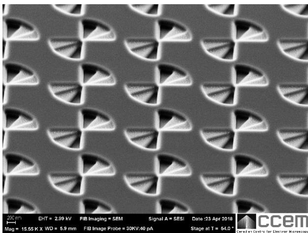
**Figure 3:** Variable-depth infrared-polarizing metamaterial
