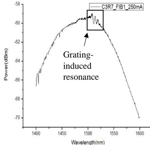
**Figure 1:** FIB-modified optical amplifier - narrow resonance band created by Bragg grating)
