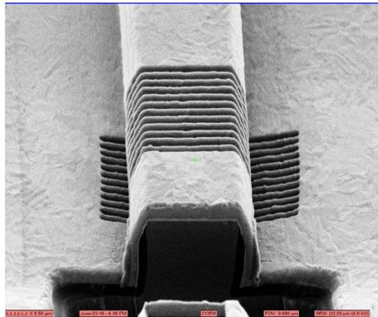
**Figure 2:** Waveguide end faceting to create DFB laser cavity
