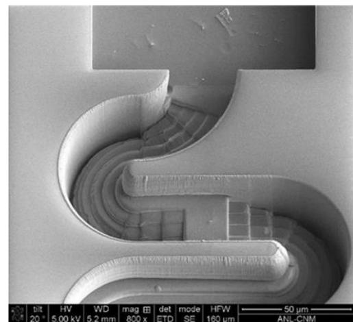
**Figure 4:** Microfluidic mixer fabricated with a multi-step process (Ocola et al)
