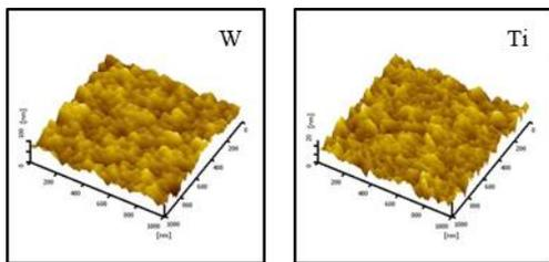
Fig.3 AFM images of the surface.
