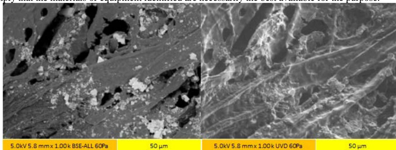
**Figure 1.** Hitachi SU5000 FE/UVD SEM images in BSE (left) and UVD (right) modes with the use of the ionic liquid HILEM IL 1000 on samples of 25% cotton paper, scale at 50.0 µm.
