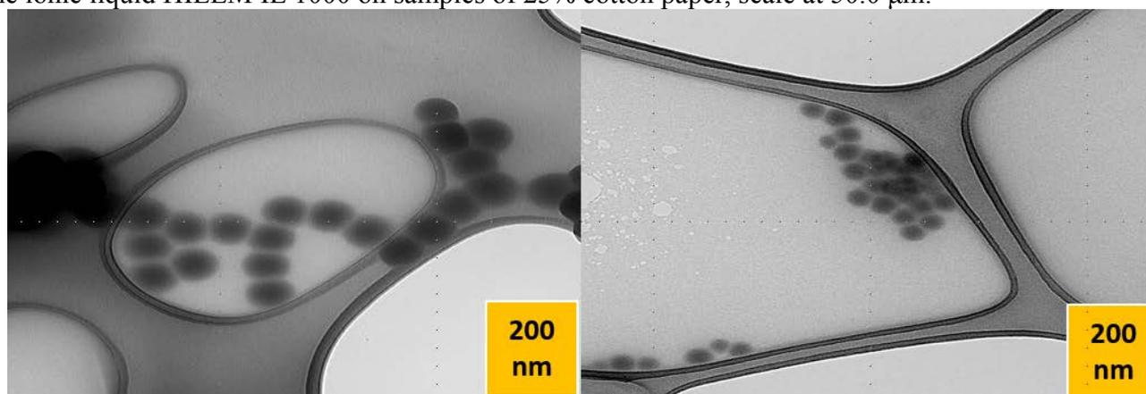
**Figure 2.** Hitachi HT7800 120 KV TEM images with the use the ionic liquid HILEM IL 1000 on SRM 1963a (left, 100 nm polystyrene spheres) and 1964 (right, 60 nm polystyrene spheres), scale at 200 nm.
