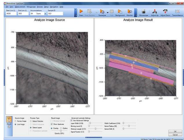
Figure 2. Detection of layers in a multilayer food packaging material
