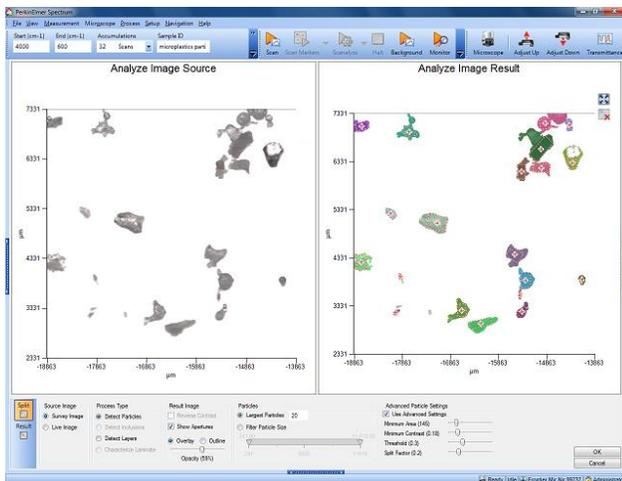
Figure 1. Use of Detect Particles to find microplastics on a membrane filter
