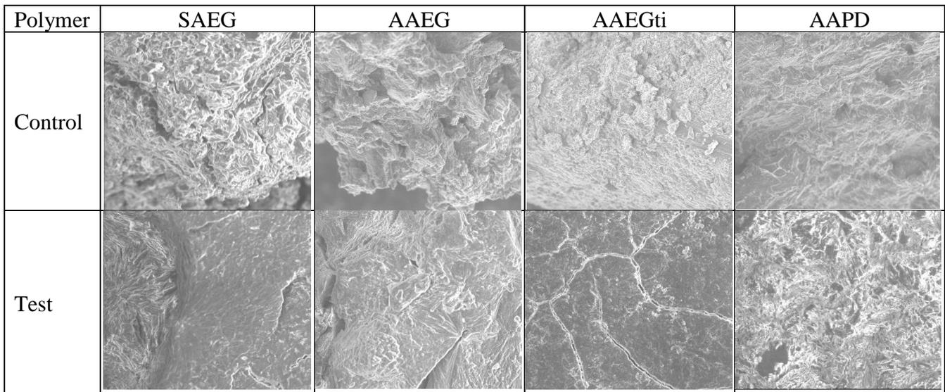
**Figure 3.** SEM viewgraphs of biopolymers buried in soil (test) or sterilized soil (control) for 60 days.
