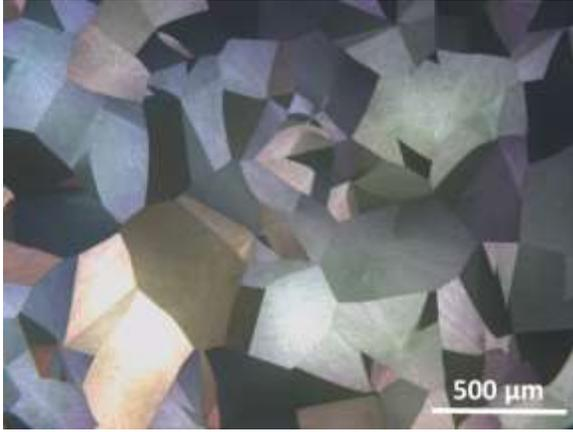
Fig. 1 Polarized optical microscopy image shows a polycrystalline structure with a grain size of about 150 $\mu\text{m}$ .
