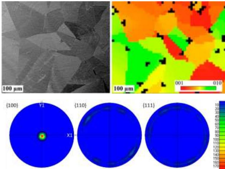
Fig. 2 (a) SEM image and (b) corresponding orientation map (inverse pole figure -X) of the same region. (c) is pole figures of the orientations obtained from map (b).
