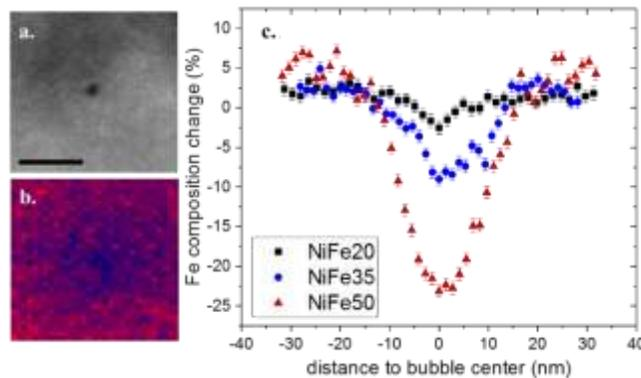
**Figure 2.** (a) HAADF-STEM image showing region where EELS spectrum image was taken. He bubble is low intensity region in center of image. The scale bar is 20 nm; (b) corresponding composition map (Ni is blue, Fe is red); (c) profiles of absolute Fe concentration changes near He bubbles in three  $\text{NiFe}_x$  SP-CSAs.
