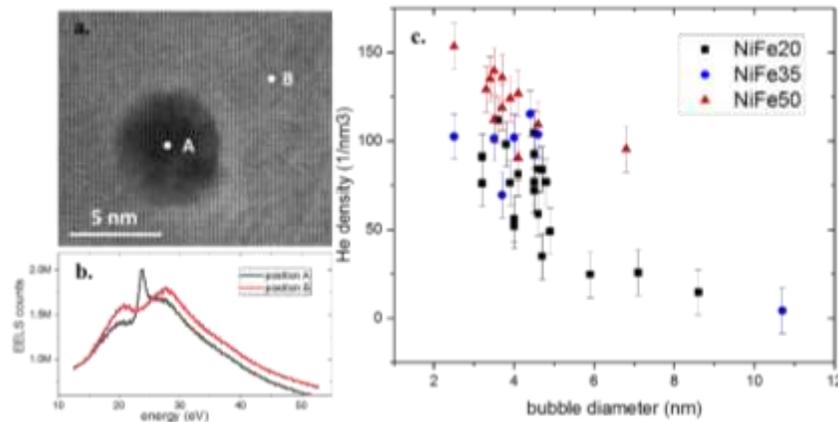
**Figure 1.** (a) HAADF-STEM image of a typical He bubble in  $\text{NiFe}_{50}$ ; (2) EELS profiles acquired from positions A and B in (a); (c) He densities inside bubbles of different sizes in three SP-CSAs.
