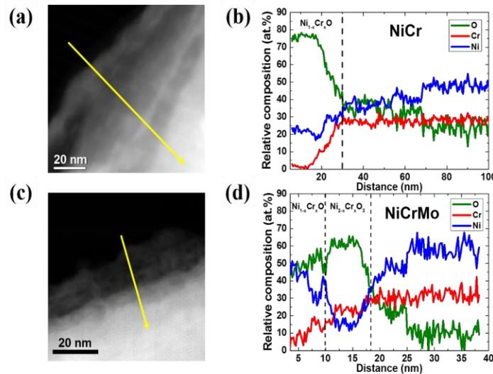
**Figure 3.** HAADF images of the oxidized samples after in-situ experiments for (a) NiCr and (c) NiCrMo samples, the yellow arrows indicate the EELS line-scanning direction. (b) and (d) are EELS relative composition profiles for Ni-Cr and Ni-Cr-Mo respectively.
