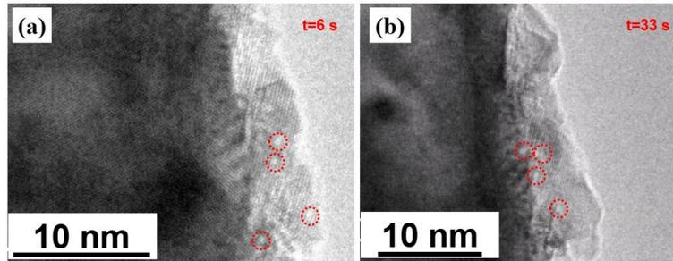
**Figure 1.** In-situ TEM images showing Kirkendall voids (dotted circles) formed (a) in the rock-salt film and (b) near the oxide-metal interface of the NiCr alloy.
