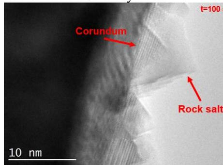
**Figure 2.** TEM image showing the corundum structure quickly formed after a couple of layers of rock-salt formation in NiCrMo alloy.
