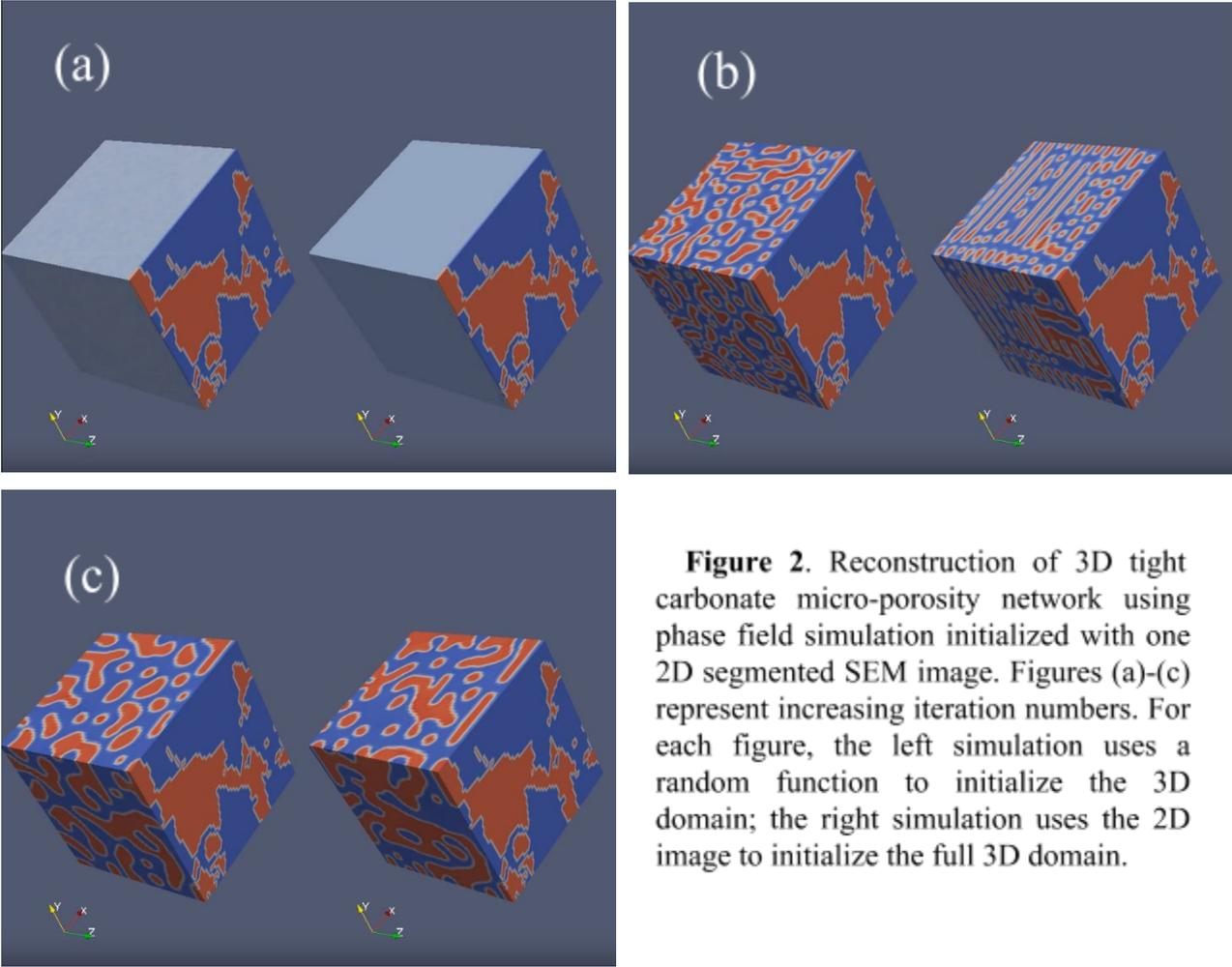
**Figure 2.** Reconstruction of 3D tight carbonate micro-porosity network using phase field simulation initialized with one 2D segmented SEM image. Figures (a)-(c) represent increasing iteration numbers. For each figure, the left simulation uses a random function to initialize the 3D domain; the right simulation uses the 2D image to initialize the full 3D domain.
