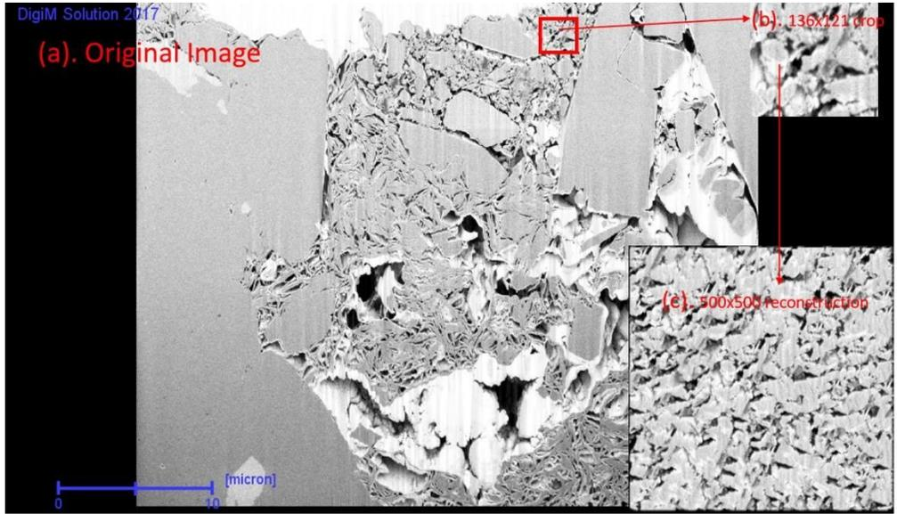
**Figure 1.** Reconstruction of tight sandstone intergranular porosity using GPU accelerated texture synthesis. (a). Original SEM image with heterogeneity and imaging artifact that made it unsuitable for petrophysical modeling; (b). Small area representative for intergranular porosity; (c). Reconstructed intergranular porosity from (b) using texture synthesis on a more representative larger area that is suitable for petrophysical characterization.
