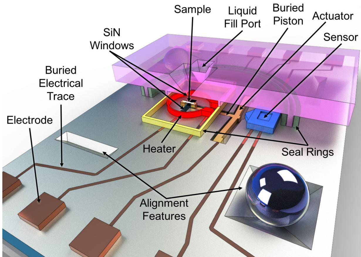
**Figure 1.** Labeled schematic of mechanical-electrical-thermal MEMS platform base.
