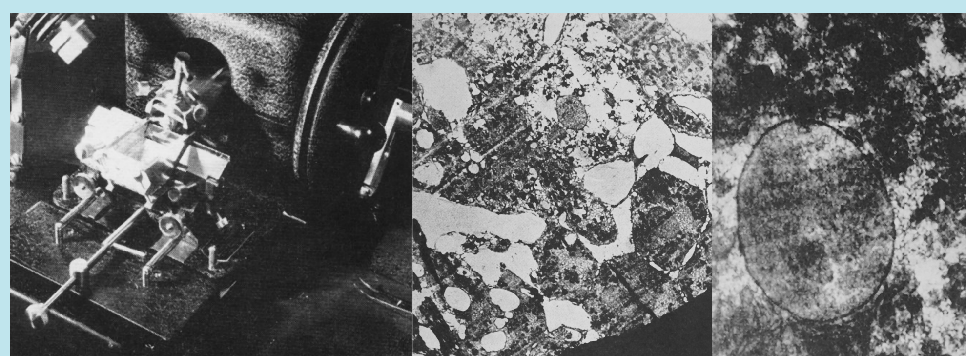
An improved ultramicrotome (Hillier and Gettner, 1950a,b). Artifacts associated with earlier ultramicrotomy work by Pease and Baker (J. Appl. Phys. 20, 480, 1949) were analyzed, and further modifications were made to a standard Spencer microtome. Cutting sections directly onto a water surface proved provide a method by which good sections could be obtained without the need to subsequently remove the embedding material. Good quality 200-nm-thick sections could routinely be obtained. Sections shown are of liver tissue.
