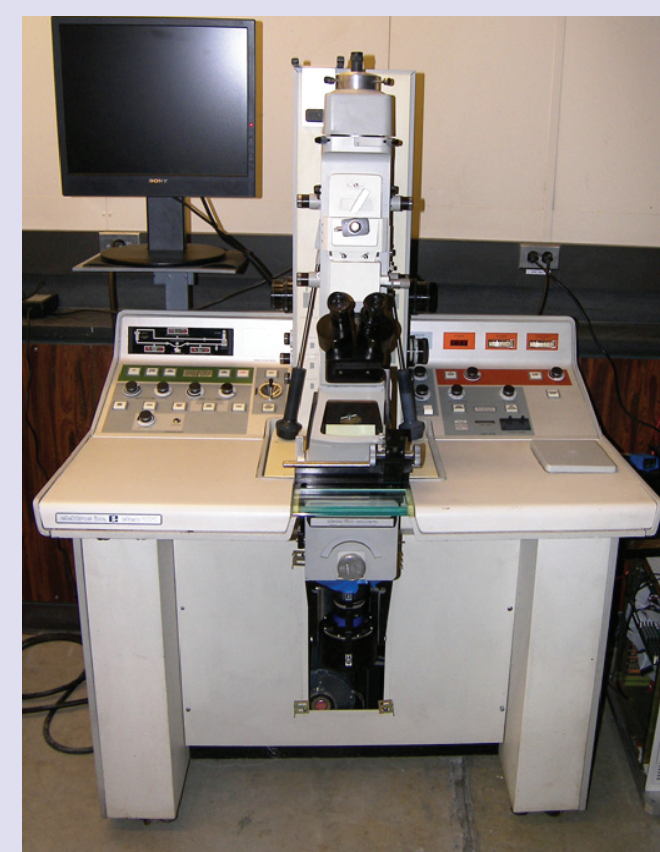
Fig. 3 An operating Elektrostat electrostatic TEM, located at Portland State University. The EM operates at 40 kV, and is completely self-contained, needing no cooling water. It has an automatic vacuum system and a real-time stereo imaging feature. (A modern CCD camera has been added).
