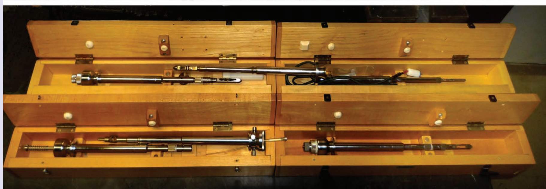
As described in a comprehensive paper (Swann, 1978) specimen holders made by Gatan for the EM-7 included heating, cooling and straining holders of both single and double-tilt configuration (most of which still exist at Albany). Note the representations of a young Peter "flying" in a holder at upper left (and "sleeping" in one at upper right in the previous figure). An early sketch of a holder tip is also shown.
